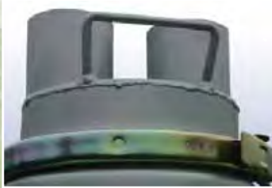
Quick Detach Inlet Quick coupled for ease of inspection and building of solid plug.
